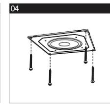
Place the speaker box close to the hole, and fix the speaker box to the ceiling, using the screws provided
