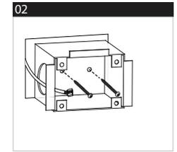
Pass the cable through the bracket hole and then fix the bracket.
