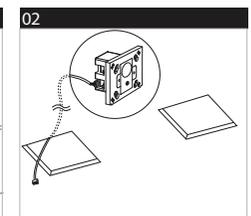
Take out the cable beforehand connected to the VOL&AUX through the hole of the one side.
