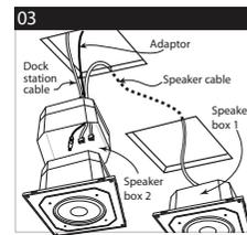
Connect the dock station, speaker cable and adaptor respectively to the connectors in the PCB board found in the compartment of the larger speaker (speaker box 2)
