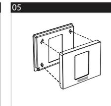
Push the cover until it snaps in place. Make sure the cover open down (as shown)
