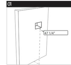
Make a 75x65mm (3" x 2-9/16") hole in the place where the dock station will be installed. **The dock station has to be installed outside the shower**
