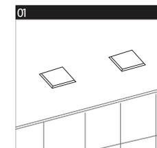
Cut two holes of 115x115mm (4 1/2" x 4 1/2") on the ceiling
